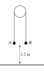
Particles A of mass 0.4 kg and B of mass 1.6 kg are attached to the ends of a light inextensible string which passes over a fixed smooth pulley. A is held at rest and B hangs freely, with both straight parts of the string vertical and both particles at a height of 1.2 m above the floor (see diagram). A is released and both particles start to move.
