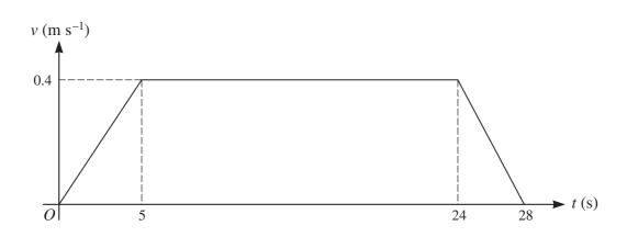
An elevator is pulled vertically upwards by a cable. The velocity-time graph for the motion is shown above. Find
