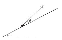
A small block of weight 5.1 N rests on a smooth plane inclined at an angle  $\alpha$  to the horizontal, where  $\sin \alpha = \frac{8}{17}$ . The block is held in equilibrium by means of a light inextensible string. The string makes an angle  $\beta$  above the line of greatest slope on which the block rests, where  $\sin \beta = \frac{7}{25}$  (see diagram). Find the tension in the string. [3]
